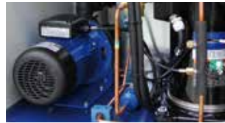
P3 (3 barg) and P5 (5 barg) pump, as optional.
